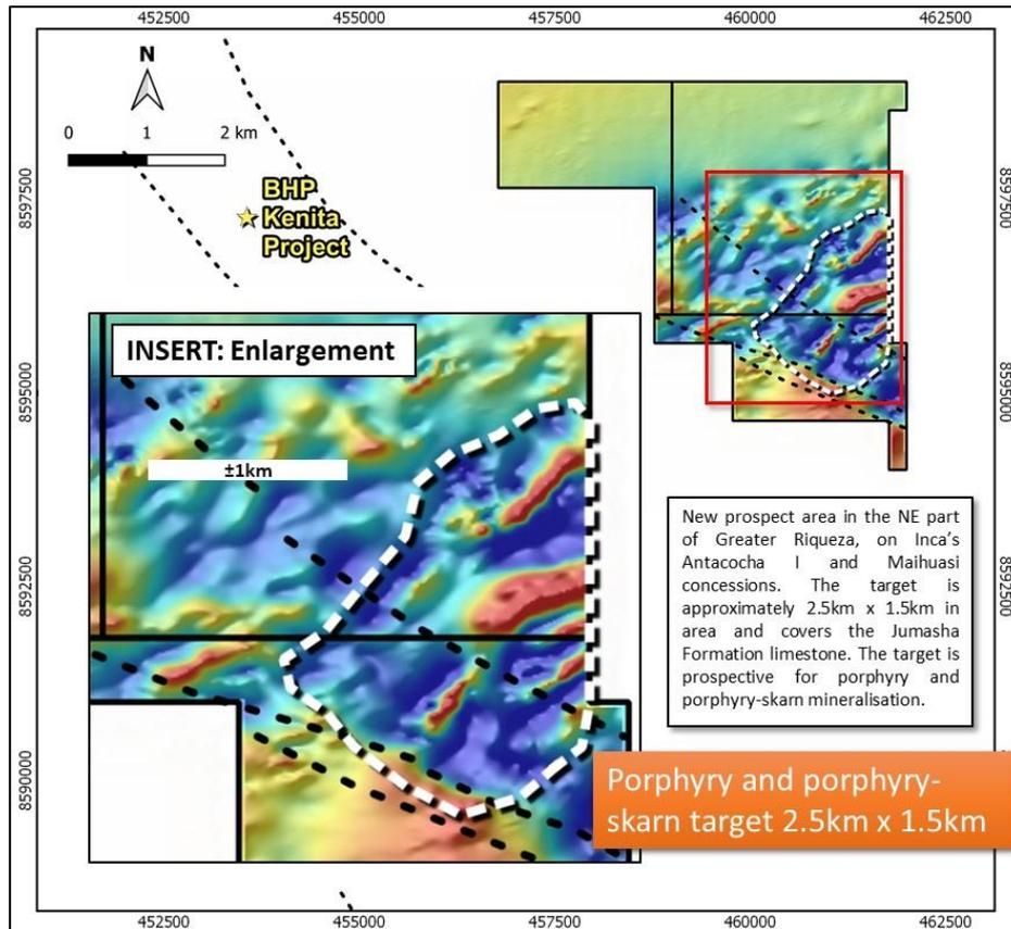
Figure 3 LEFT: A preliminary TMIRTP image showing raw, gridded total magnetic intensity data reduced to pole providing a basic level of interpretation. Highlighted is the Yanacolipa porphyry and porphyry-skarn target-centre
