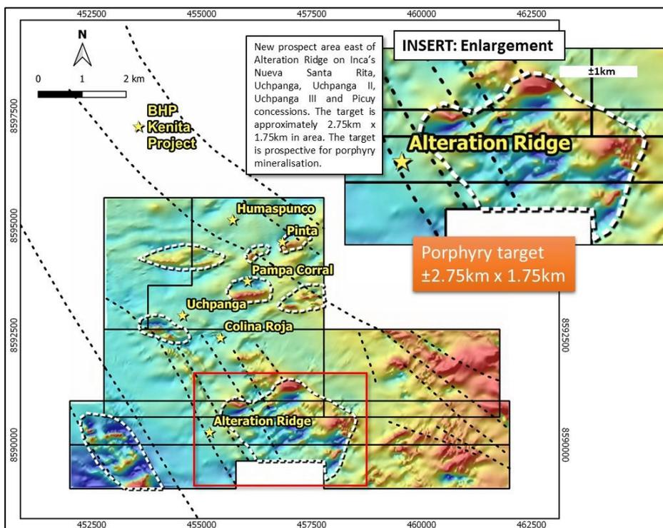
Figure 2 **LEFT**: A preliminary TMIRTP image showing raw, gridded total magnetic intensity data reduced to pole providing a basic level of interpretation. Highlighted is the Palcacandha porphyry target-centre.
