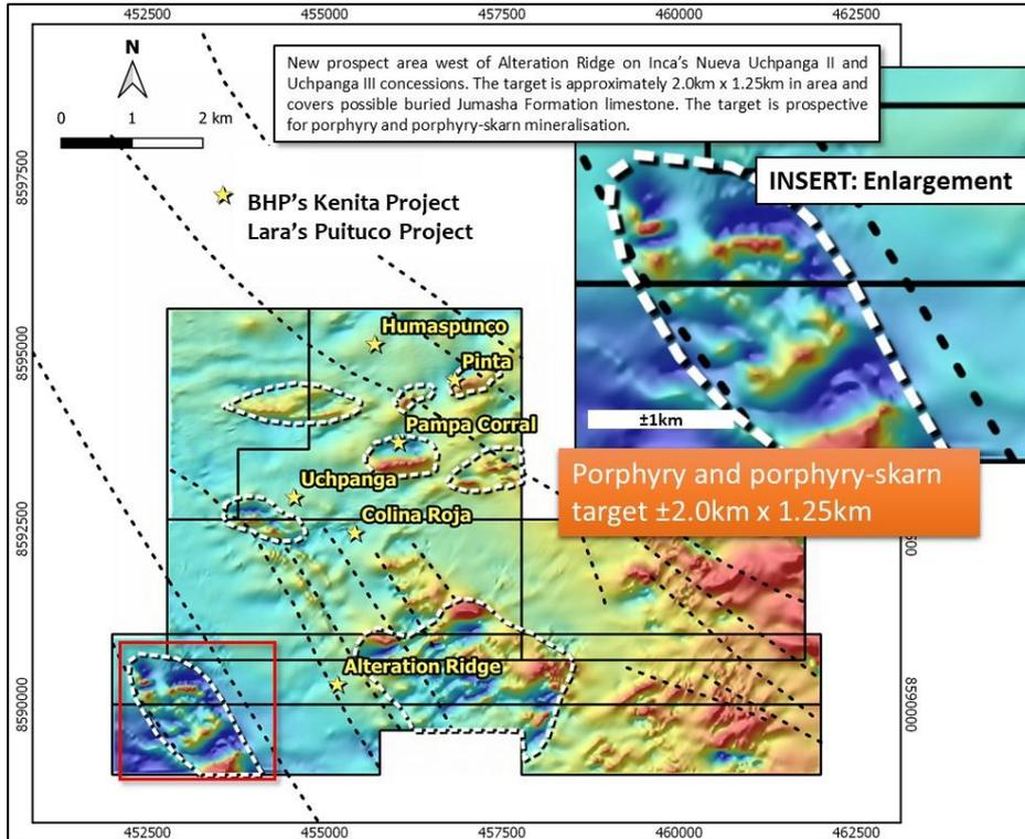
Figure 1 **LEFT**: A preliminary TMIRTP image showing raw, gridded total magnetic intensity data reduced to pole providing a basic level of interpretation. Highlighted is the Tayapampa porphyry and porphyry-skarn target-centre.
