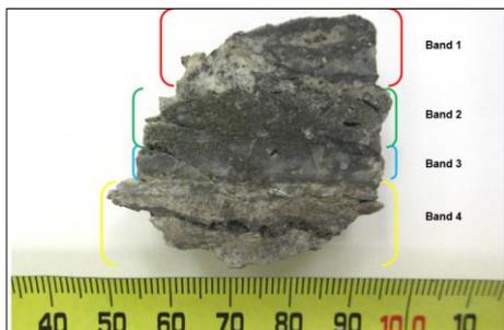
Figure 5: **LEFT** Vein material from the Rita Maria working at the western end of Uchpanga. Originally a chert, the rock specimen has four recognisable bands, Band 1: chert with galena, sphalerite, stibnite (antimony sulphide) and barite; Band 2: Quartz with pyrite and sphalerite; Band 3: Recrystallised quartz vein with sphalerite; and Band 4: Quartz with clays. Material such as this in previous sampling by Inca has returned plus-gram per tonne gold and bonanza grade silver.
