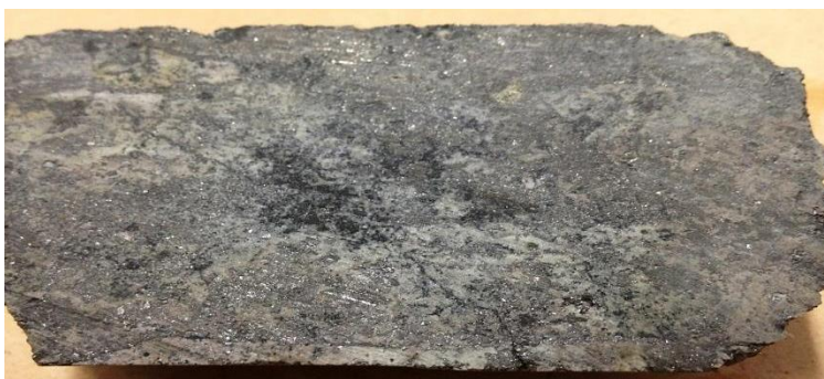
Figure 2: Core photo at 74m CH-DDH005: Tourmaline breccia with pyrite veining and disseminated sulpho-salts as breccia matrix material. INSERT: Distinctive zoned pyrite veinlet with detail of highly altered volcanic. The interval from 73m to 75m contains 0.95g/t Au, 14.15g/t Ag.
