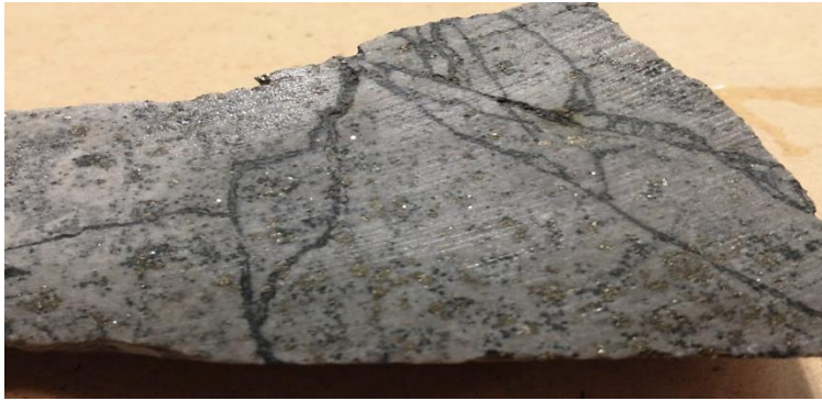
Figure 4: Core photo at 72.5m CH-DDH005: Highly altered volcanic with blebby pyrite and tourmaline/sulphide veinlets. The interval from 72m to 73m contains 0.76g/t Au, 12.3g/t Ag and 0.11% Cu as well as elevated Pb and Zn.
