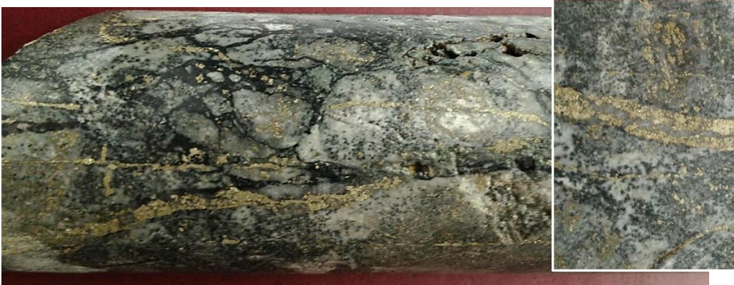
Figure 2: Core photo at 74m CH-DDH005: Tourmaline breccia with pyrite veining and disseminated sulpho-salts as breccia matrix material. INSERT: Distinctive zoned pyrite veinlet with detail of highly altered volcanic. The interval from 73m to 75m contains 0.95g/t Au, 14.15g/t Ag.
