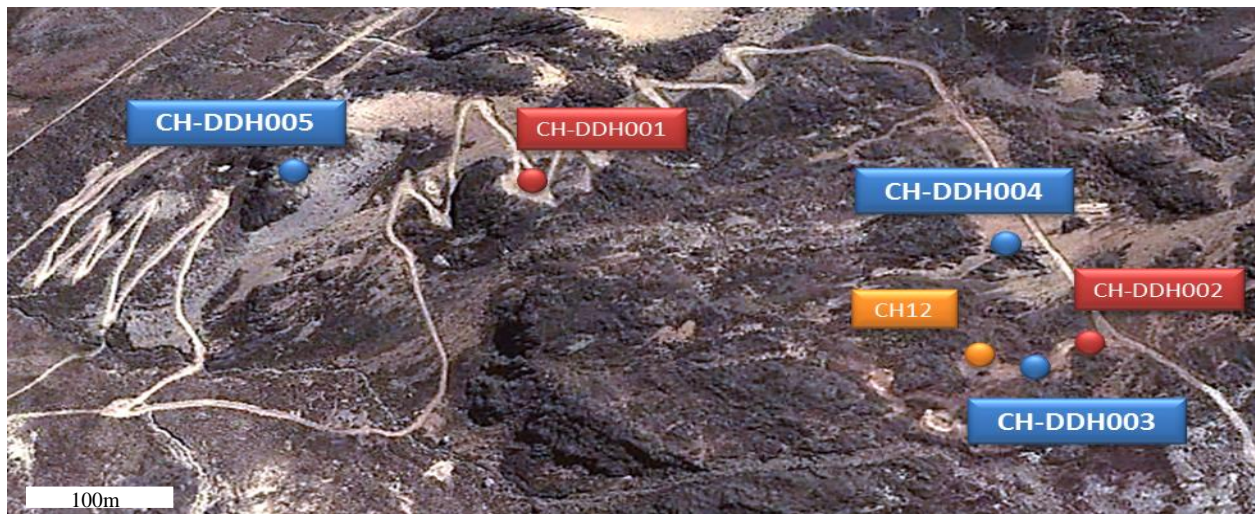
Figure 1: Location plan of Inca's drill holes at Chanape. BLUE: Recently completed holes by Inca. RED: Inca's “discovery” hole CH-DDH001, which intersected shallow gold/silver mineralisation in Breccia Pipe 8 and mineralised porphyry at 380m; CH-DDH002, which intersected shallow gold-silver bearing “crackle breccia”. ORANGE: Drill hole completed by a previous company, which also intersected shallow gold-silver mineralisation.
