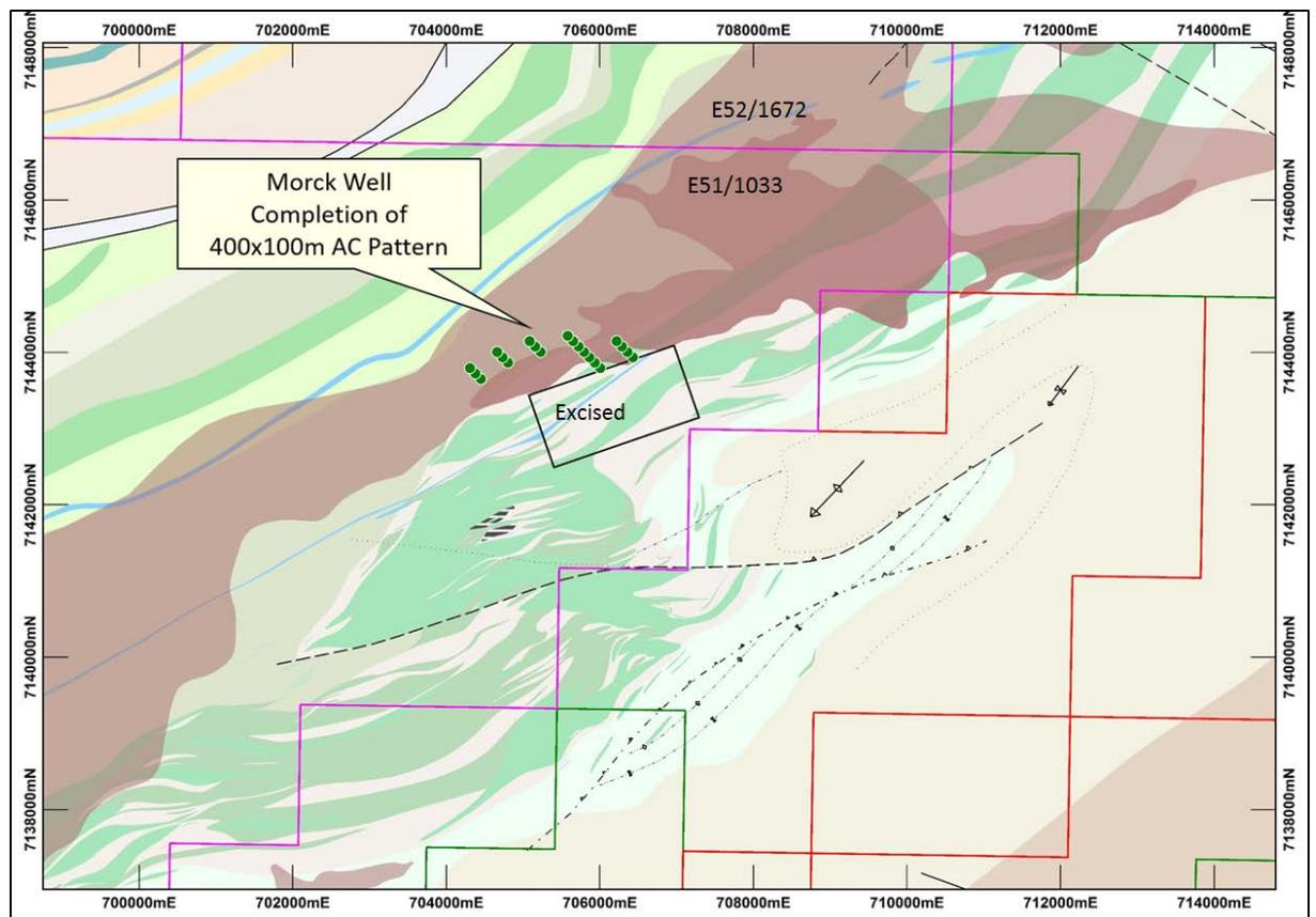
**Figure 4. AC Drilling conducted within the Morck Well Project during Q1, 2019 (Auris Tenements labelled with pink outline)**
